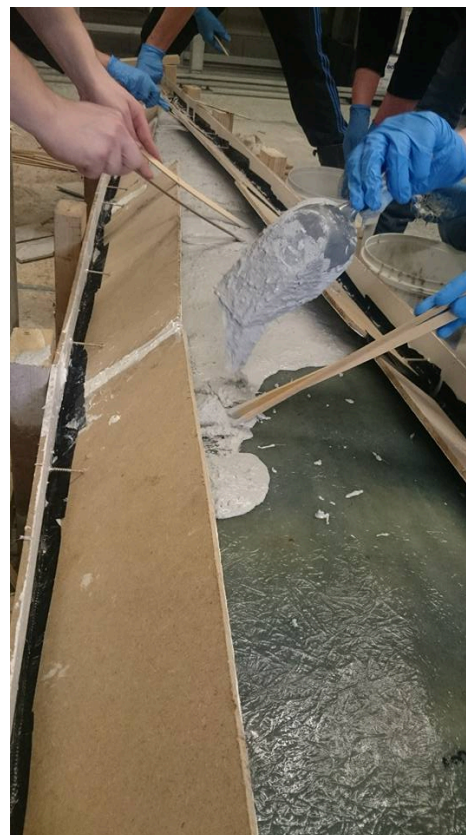
Figure 20: Pouring the floor of the canoe
