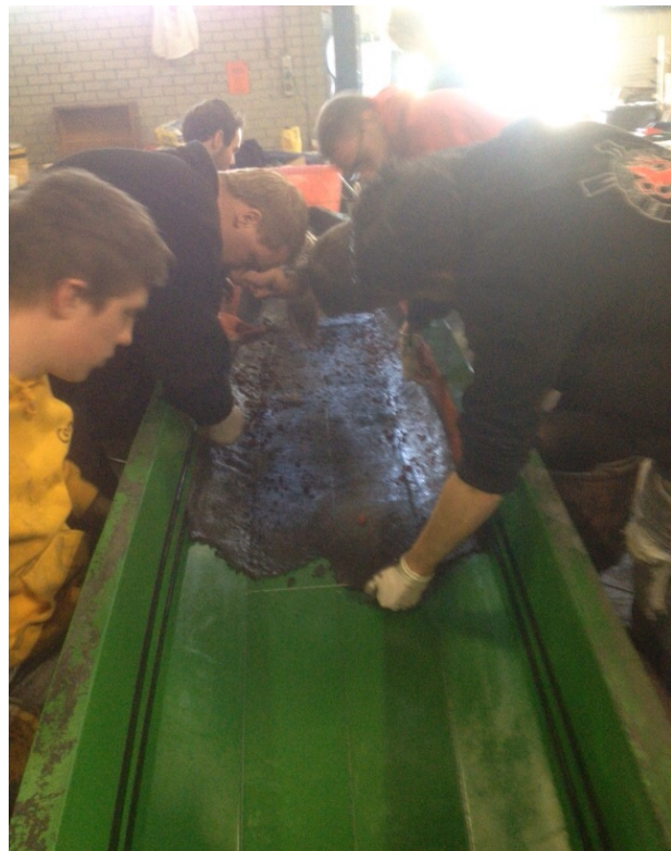
Figure 17: applying the concrete to the canoe
