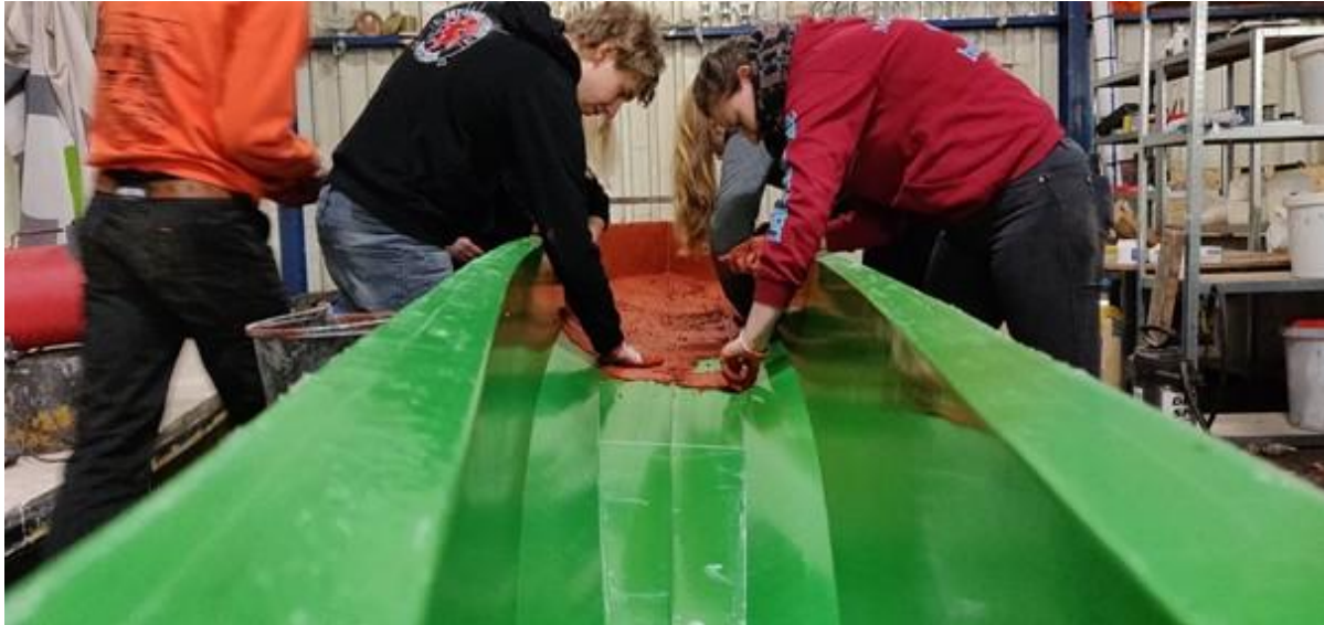
Figure 2: Applying the first layer of concrete to the mould.
