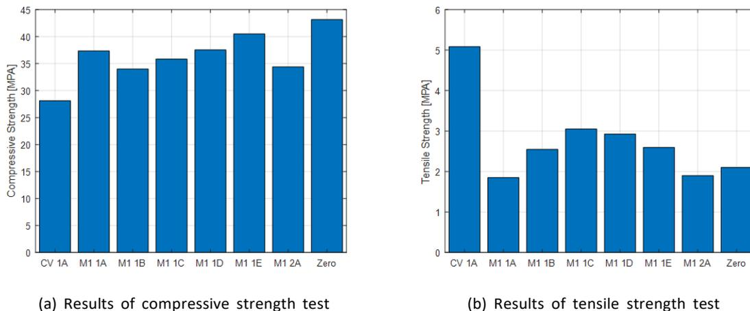
Figure 3: Results of laboratory tests
