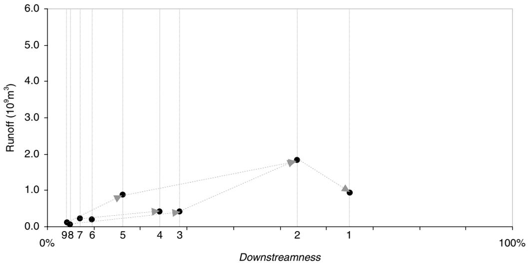
**Fig. 7.** Average annual runoff at selected locations 1–9 characterized by their downstreamness for 1996–2008; arrows indicate direct connections of measurement locations through the river network
