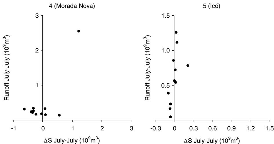
**Fig. 6.** Comparison of upstream storage and annual runoff at two measurement stations in the Jaguaribe Basin; change in stored volumes and runoff for annual time periods, similar to Fig. 1; storage capacity upstream of Measurement Station 4 (Morada Nova) is relatively large (see Table 1), possibly associated with major closure; the storage upstream of Measurement Station 5 (Icó) is relatively small (see Table 1), possibly associated with minor closure
