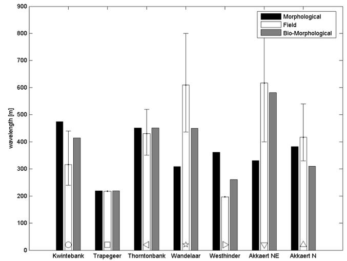
Figure 6. Comparison between the predicted and measured wavelength of the sandwaves at the different sites for both the morphological model (Cherlet et al., 2007) and the bio-morphological model. Markers at the bottom of the plot correspond to the markers used in Figure 4.
