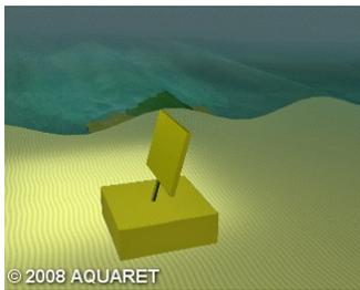
Figure 8.3: Oscillating wave surge device
