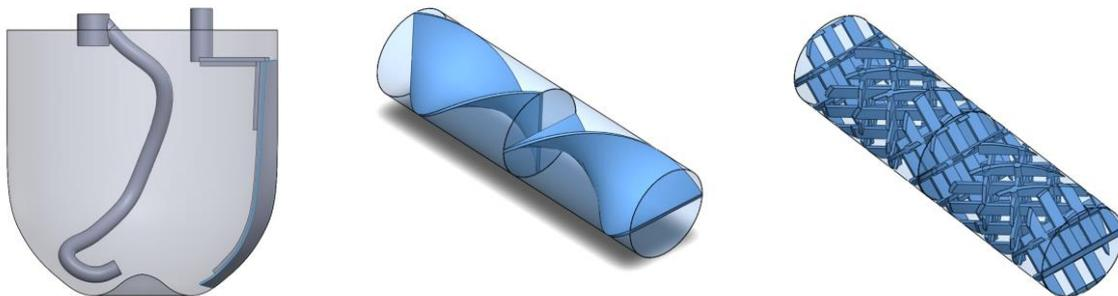
Figure 1: Dough mixer, helical static mixer and x-grid static mixer
