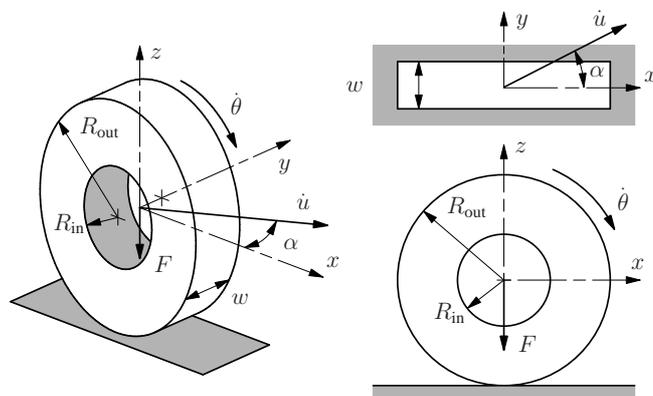
Figure 1 : The small test tyre.
