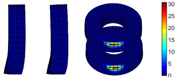
a Deformed shape for explicit solver (right) and Abaqus/Explicit. b Shear force in N for explicit solver (above) and Abaqus/Explicit
