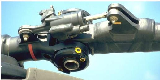
Figure 1 : External view of a lag damper
