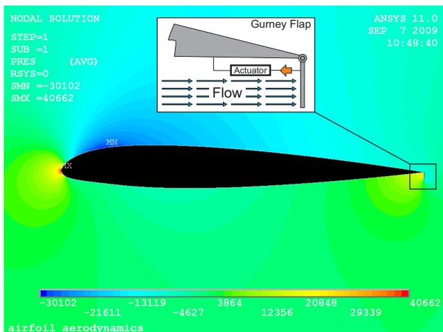
Figure 1 : Pressure distribution around Naca 23012 airfoil with a 2% chord length Gurney flap at the trailing edge.
