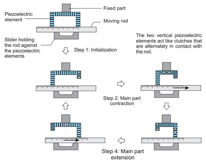
Figure 2 : Working principle of a stepped actuator.
