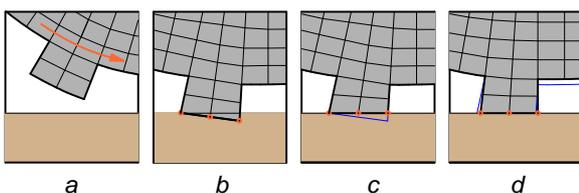
Figure 1 : Simplified working of the contact algorithm: a tread block (a) is displaced under the road (b), is put back on the road (c) and is corrected for slip (d).
