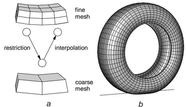
Figure 3 : Multigrid cycle (a) and coarse tyre mesh (b)
