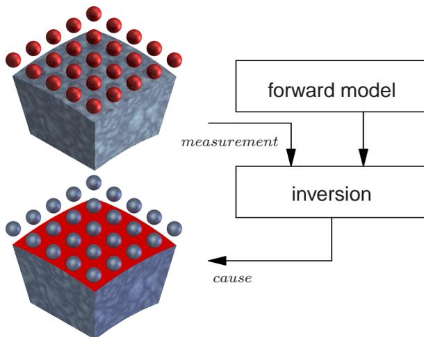
Figure 1 : inverse acoustics. Spheres: acoustic sensors.
