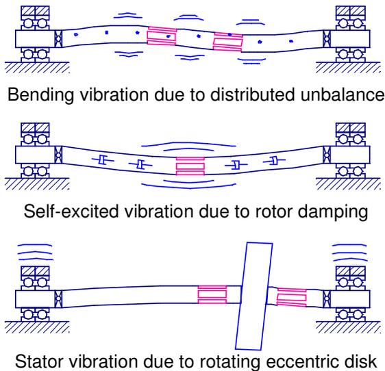
*Fig.1. Typical rotor dynamic problems (actuators in red).*
