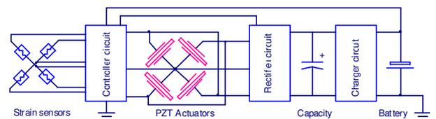
*Fig.3. Circuit diagram of a self-powering balancing device*
