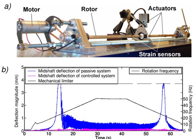
*Fig.2. Deflection magnitudes for shown rotor setup.*
