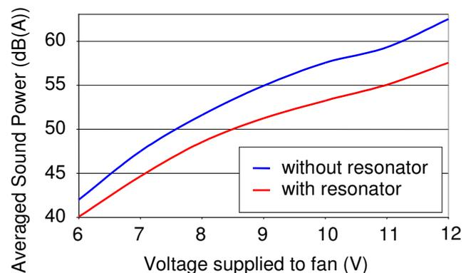
Fig. 4) Sound power measurements of the demonstrator
