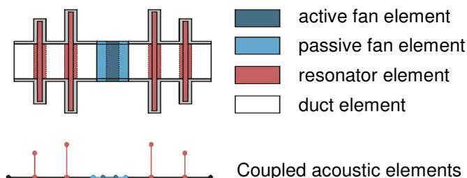
Fig. 2) Schematic overview of a multi resonator setup
