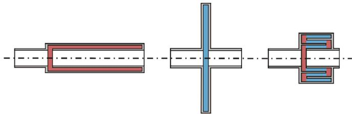
Fig. 1) Cylindrical, circular and folded resonator geometry
