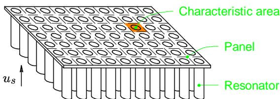
Figure 2 : Part of a panel with acoustic resonators
