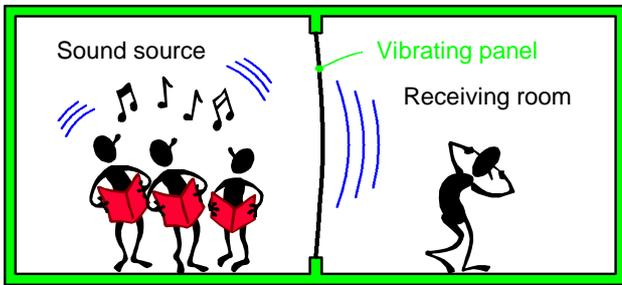
Figure 1 : Sound transmission between two rooms
