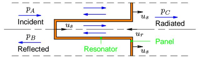
Figure 3 : Normal incidence transmission of sound through a characteristic area
