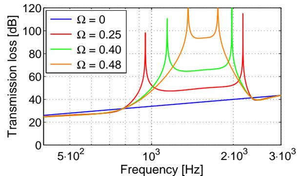
Figure 4 : Normal incidence sound transmission loss for different porosities
