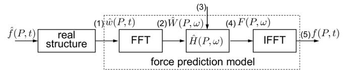
Figure 2 : Direct Inverse Method, frequency domain
