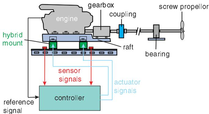
Figure 1 : Hybrid isolation of a ship engine (TNO)
