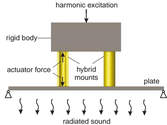
Figure 2 : Model of a hybrid isolation structure
