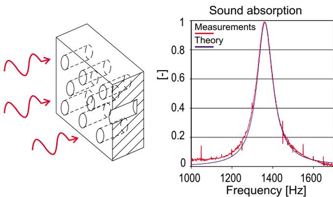
Figure 1. Optimized sound absorbing wall.
