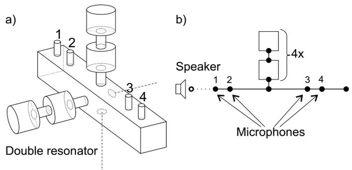
Figure 4. Experimental (a) and numerical (b) set-up with Helmholtz resonators.
