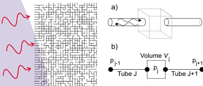
Figure 2. Network of tubes to model sound absorbing material.
