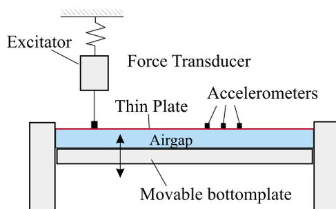
Figure 2 : Experimental setup
