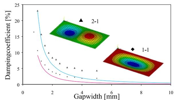
Figure 4 : Damping as a function of gapwidth
