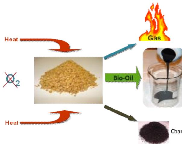
A schematic of flash Pyrolysis of Wood
