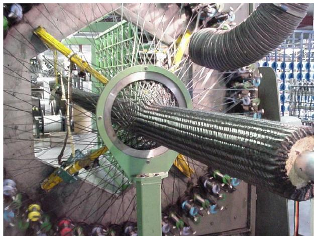
Figure 1: Overbraiding (Courtesy Eurocarbon).
