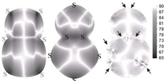
Fig 4: Simulation results,  $[0^\circ/90^\circ]_{2s}$ ,  $[45^\circ/-45^\circ]_{2s}$  and QI lay-up
