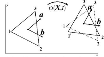
Fig 2: Remap of the fibre orientations from deformed ply onto the average deformation
