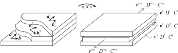
Fig 1: Individual and averaged ply deformations of a three layer laminate
