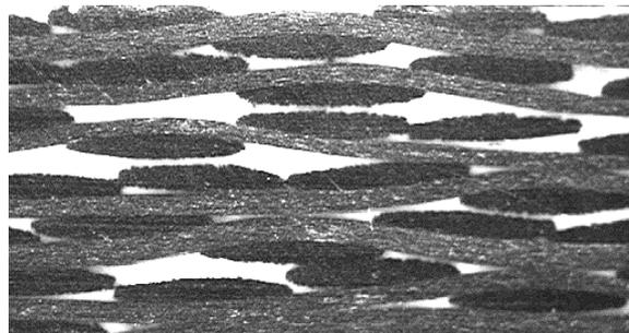
*Fig.1 Microscopic image of a cross section of an undamaged 0/90° woven fabric reinforced PPS laminate*
