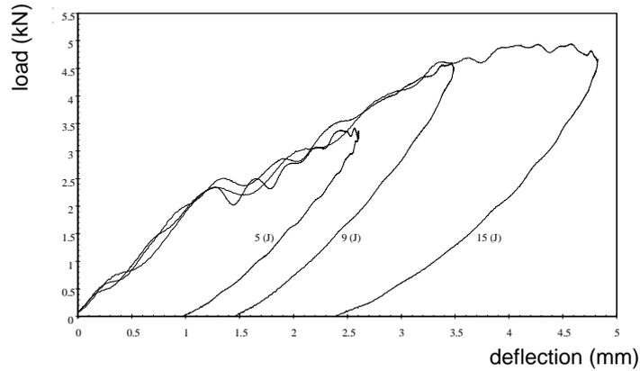
Fig. 3 Load-deflection curves from IFWIM experiments at 5,9,15 J incident energies.
