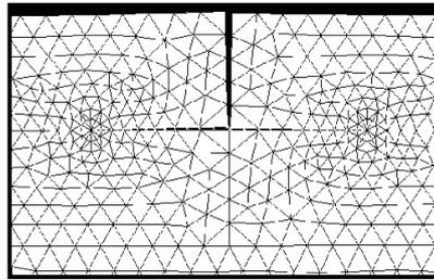
Fig. 5 Detail of the FE mesh for the analysis of delamination growth in the presence of a transverse crack.
