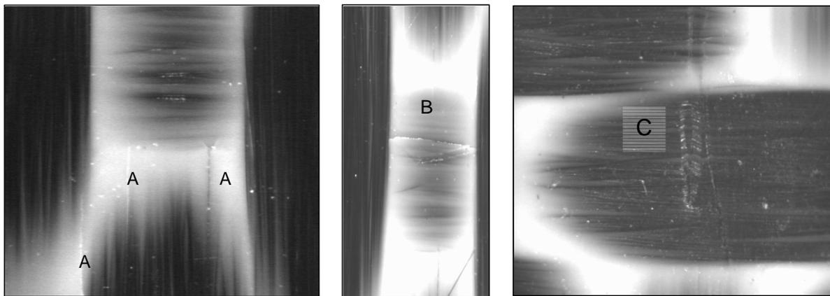
*Fig. 2 Damage initiation in quasi-static beam bend tests; A: transverse cracks in the predominate  $90^\circ$  yarns on the tensile face; B: transverse cracks in the  $0^\circ$  yarns on the tensile face; C: microbuckling in the predominate  $0^\circ$  yarns on the compressive face.*
