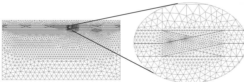
Fig.4 Finite Element mesh of a fabric layer with a tilted interyarn crack, with homogeneous material outside the layer.
