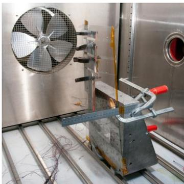
*Measurement setup to measure bow in a temperature controlled environment*
