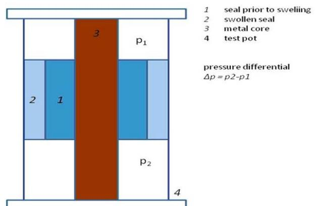
Fig. 1 Schematic view of PIT-unit for pressure testing of seals at temperatures up to 300°C and pressure differentials of 150 bar.
