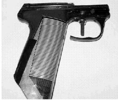
**Figure 2.** The sensor wrapped around the gun’s butt.
