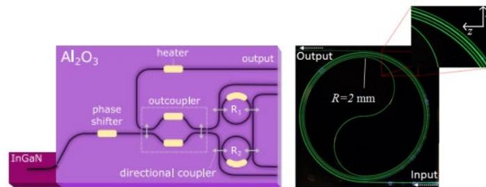
Figure 1 Hybrid integrated near UV lasers [2] On-chip Er<sup>3+</sup>:Al<sub>2</sub>O<sub>3</sub> spiral amplifier [3]
