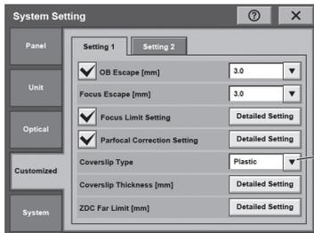
**TIP** Set the material (glass or plastic) of the bottom of the specimen container to be used.
