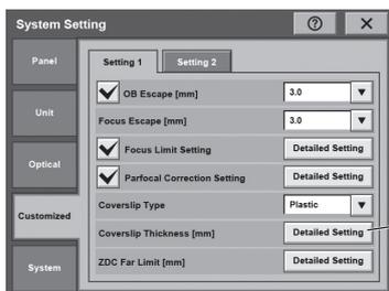
**TIP** Set the thickness of the bottom of the specimen container to be used for each material (glass or plastic).
