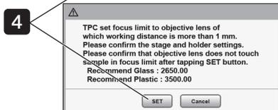
**TIP** For an objective that does not (cannot) use the recommended value, set the focus limit individually.
