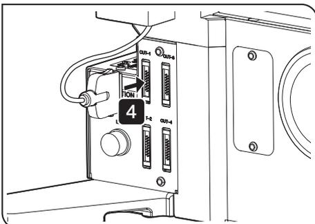
**4** Connect the cable connector of the Z drift compensator to the connector of the microscope frame.
