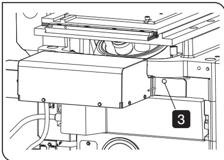
**3** While keeping the Z drift compensator pushed in, tighten the clamping screw of the Z drift compensator using the Allen screwdriver provided with the microscope frame.
