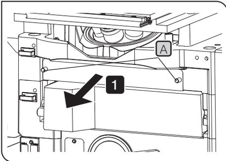
**1** Remove the clamping screws **A** and remove the cover of the microscope frame.
