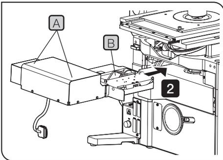
**2** Hold the top and bottom parts indicated in the figure by the lines **A** in both hands, and insert the Z drift compensator to the microscope frame until it touches the end completely.
