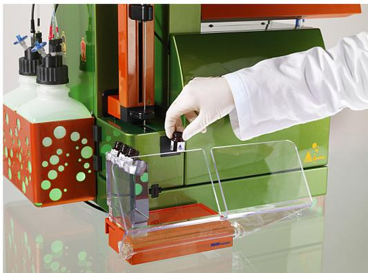
**Figure 3.3:** Enter reagents using the 2D code reader.
