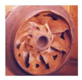
With the current commercially numerical CFD tools it very well possible to predict the effect of cavitation on the pump performance. However, to predict the erosion rates on the pump impeller surfaces currently in the pumping industry still 1D empirical models are used in which the length of the cavitation sheet is one of the major parameters.
