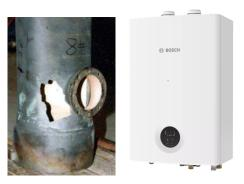
Figure 1: Left: damage to a burner liner. Right: a Bosch condensing boiler.
