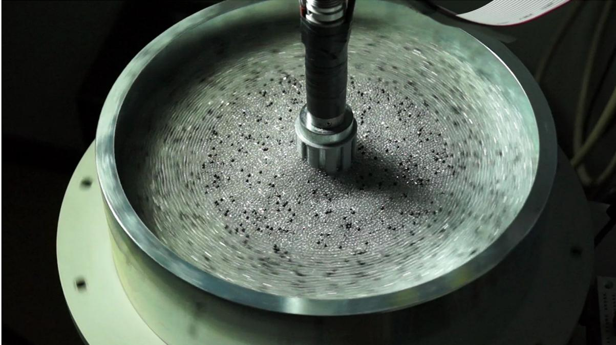
*Figure: By measuring the torque in a split-bottom shear cell, we deduce the rheological properties of wet granular materials.*
