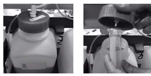
Figure 2 Manual waste collection from the CellSearch Autoprep by unscrewing the top from the waste container (left) and collecting the sample in a 50 mL Greiner tube.
