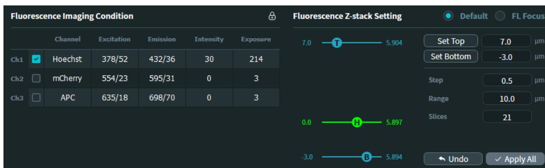
**Figure 5.6 Fluorescence setup panel (imaging conditions and Z-stack settings)**
