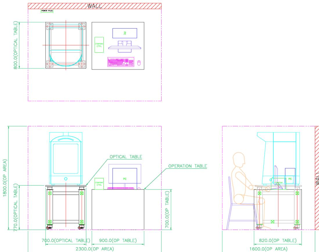
The instrument needs at least 5 cm (2 in) of clearance on each side to prevent overheating of the electronic components. Place the instrument on a level surface away from other laboratory equipment that can cause vibration of the instrument during image acquisition.
