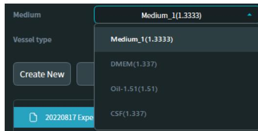
**Important!** The value for the medium RI is critical in image processing of raw image data acquired by the HT-X1. Choose a proper medium RI value before starting the image acquisition.
