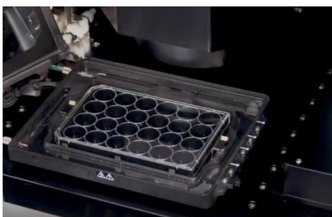
**Important!** Make sure that the dish or microplate is firmly attached to the vessel holder without tilting.
