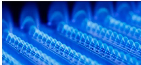
Figure 2: Laminar lean flames in slot burner.
