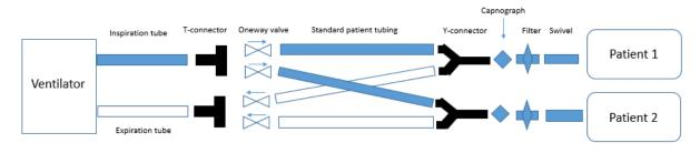
Figure 6 Schematic set-up. The arrows on the T-connectors indicate the direction in which airflow is unobstructed; airflow in the other direction is blocked. See supplement 1 for this figure in more detail and for an option without T-connectors with build in one-way-valve.
