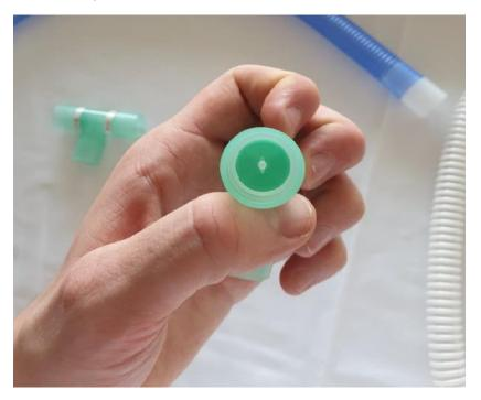
Figure 9 Inside view of T-connector, valve visible. In this direction the airflow is obstructed.
