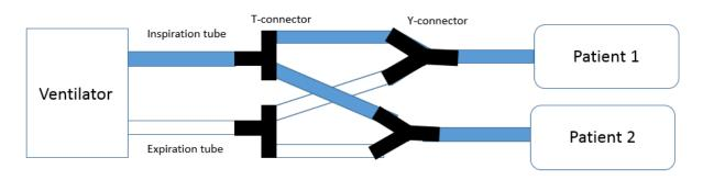
Figure 2 Schematic view how to attach 2 patients to 1 ventilator. One-way-valves are not shown in this figure
