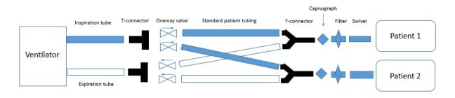
There are 4 one-way-valves required for a circuit with two patients. It is extremely important to verify that the one-way-valves are positioned in the right direction. The circuit should be tested with test lungs before connecting patients.
