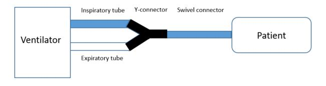
Figure 1 Standard set-up for invasive mechanical ventilation
