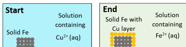
Figure 4: Microlevel representation of the redox reaction between the iron nail and the solution of copper(II)nitrate at the start and the end of the experiment.
