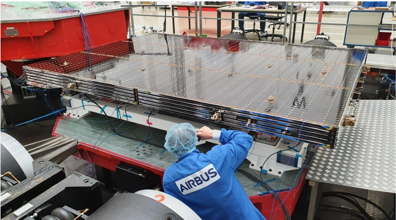
Figure 3: Solar array on the slip-table during a vibration test.
