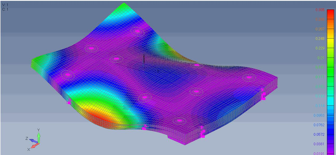
Figure 2: Typical eigenmode of the Solar Array wing in stowed configuration
