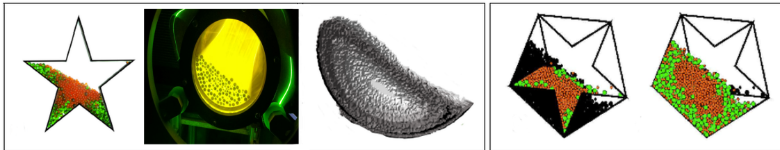
Figure 1: From the left: 1) the pattern formed inside a rotating quasi-2D pentagon drums. 2) RIMS scan of a 3D drum. 3) PEPT data for the occupancy of large particles in a rotating circular drum. 4) Simulations for the axially inhomogeneous, layered drum after four revolutions, from the front i.e., the pentagram-shaped side, and from the back the pentagonal side. Particles are coloured by size with orange small and green big; black particles correspond to those particles that belong to the opposite side of the drum.
