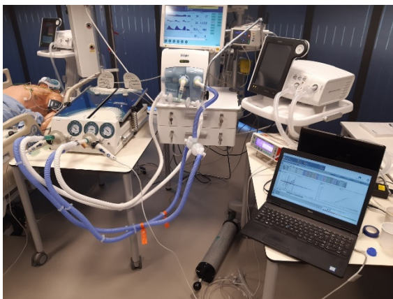
Figure 2: Set up, with a Draeger ventilator, two Fisher and Paykel tubing sets and two Vyntus Spiro PC pneumotachs, measuring the tidal volume delivered to each "patient".
