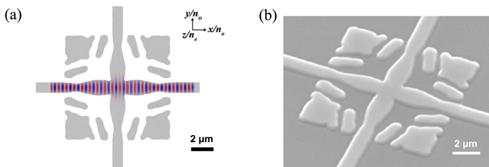
Figure 2 Example of a building block (waveguide crossing) that has been optimised using inverse design methods [4]
