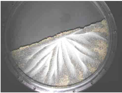
Figure 1: Mixing of different materials by using of drum.
