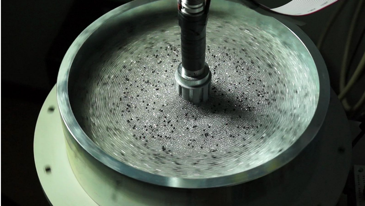
Figure: By measuring the torque in a split-bottom shear cell, we deduce the rheological properties of wet granular materials.
