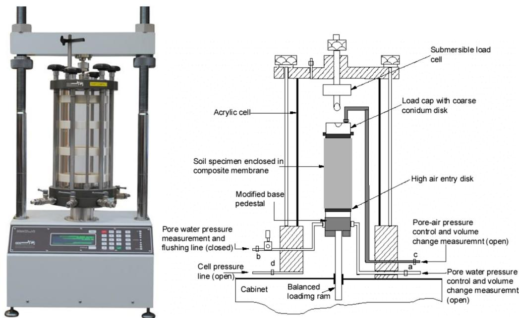
Figure 1: Triaxial cell picture and schematic.
