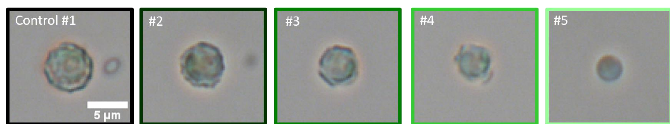
Figure 1: Optical images showing changes in the exoskeleton, due to different acid treatments. The amount of added acid increases from left to right, creating treatments with a varying range of calcification levels.
