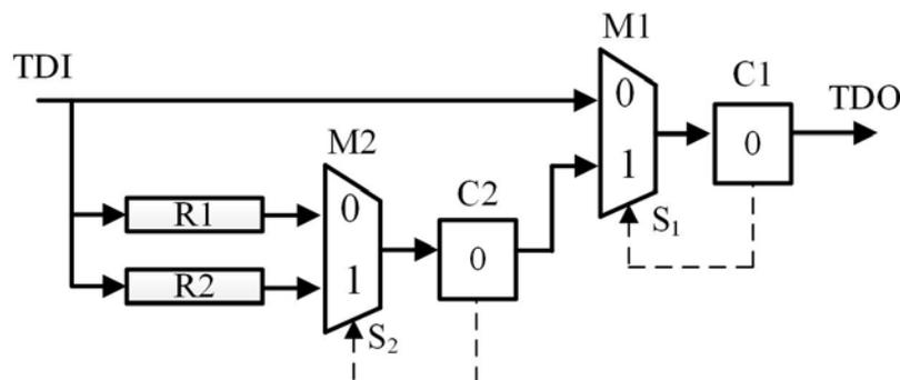
Figure 1. An RSN with two instrument ScanRegisters (R) and two network configuration ScanRegisters (C) and two ScanMuxs (M).
