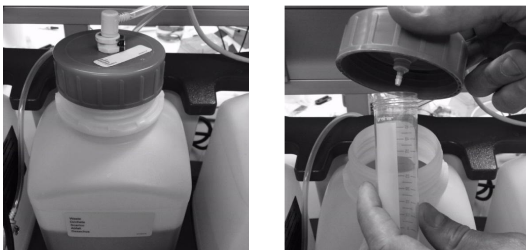
Figure 1 Manual waste collection from the CellSearch Autoprep by unscrewing the top from the waste container (left) and collecting the sample in a 50 mL Greiner tube.
