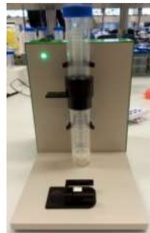
Figure 1 Complete filter tube and sieve in the filtration station. Correct filtration pressure shows a green light in the corner.
