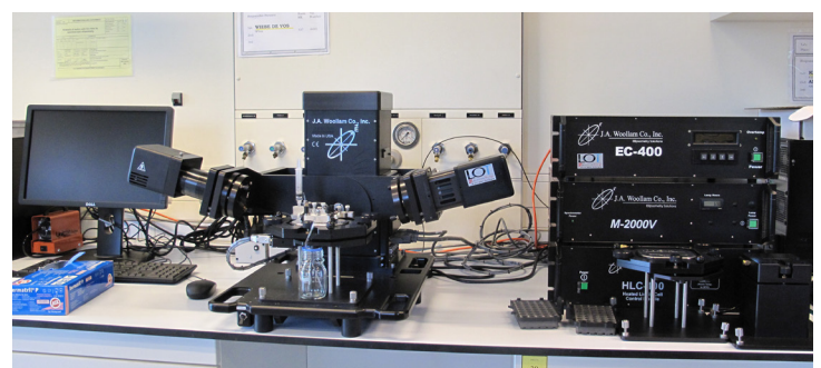
Figure 4. Photograph of the ellipsometer in our lab.
