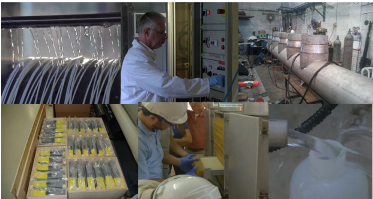
The different stadia left upper corner and then clock wise: production of the support fiber; applying the selective coating (EMI, the Netherlands), construction of the pilot (Yodfat, Israel), shipment of the modules (CUT, Germany), pilot testing (IEC, Israel) and captured water.
